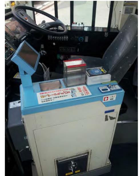
Fare box install beside the exit inside the bus to collect the fare , the driver collect the fare.
