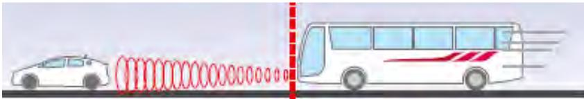
The laser radar sensor of apparatus monitor the distance to preceding vehicle .
