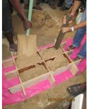
Mud concrete blocks can be manufactured at household level, using available gravel and soil mixed with cement (about 5% - 8%). The selection of appropriate soil is important in preparing high quality blocks. Soil containing gravel, commonly found in the North, is considered suitable. However, the composition of native soil can be adjusted by adding gravel, sand or clay to reach the suitable proportion.
